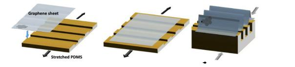
**Figure 1 :** Fig. demonstrating the process of setting graphene sheet onto textured polymer with a given stress, then releasing said stress to have the structure subdue periodic folds.
