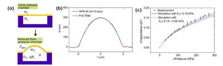
Figure 1: (a) 2-d schematic crosssection depicting the micro-blister inflation testing procedure with a single cavity and actuating membrane with significant labelled. (b) parameters 2-d topographical line profile of inflated 45 nm thick GPH micro-
