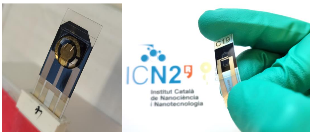
Figure 1. Examples of the electrochemical platforms produced using consumer inkjet printers and metal nanoparticles inks
