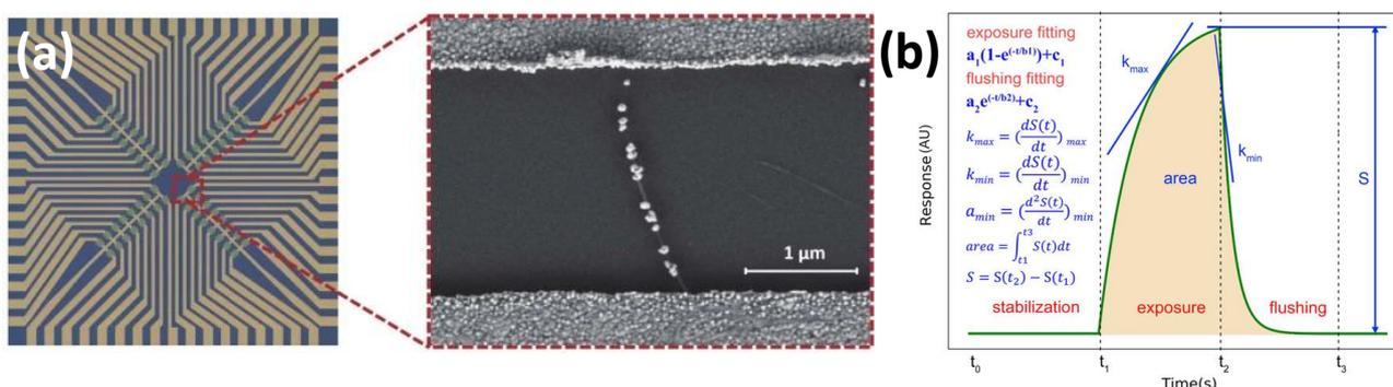
**Figure 1:** (a) Array of chemiresistors based on gold nanoparticle-modified CNTs. (b) Analysis of the interaction kinetics during exposure of sensors to a gas.
