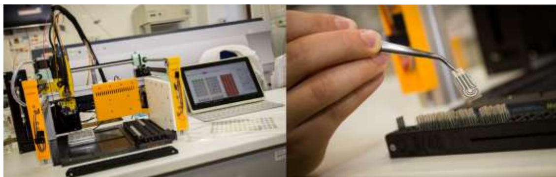
Figure 1. Fully automatic bench-top device for testing of SPEs driven by a tablet PC with user friendly SW (on left). SPEs in specially designed container preventing scratching of the active side and pins of the SPEs (on right).
