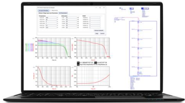
Figure 1: QuantumPro simulations, including both thermal and quantum noise effects, can be used to design cryogenic signal lines for highly scalable QPUs [1].
