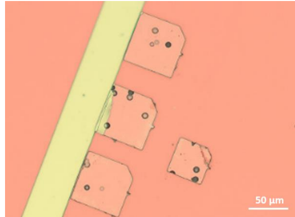
Figure 1: Example of diamond platelets bonded to a Bragg mirror next to a gold strip line for microwave delivery.
