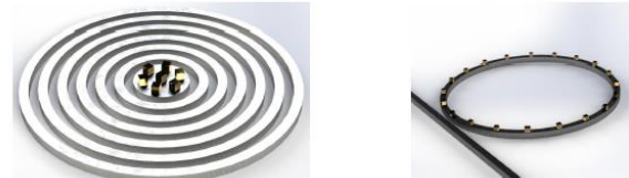
Concept of CBG and Microring resonator with distributed plasmonic nanocubes matching phase of propagating mode. Courtesy: Kryvobok, A.
