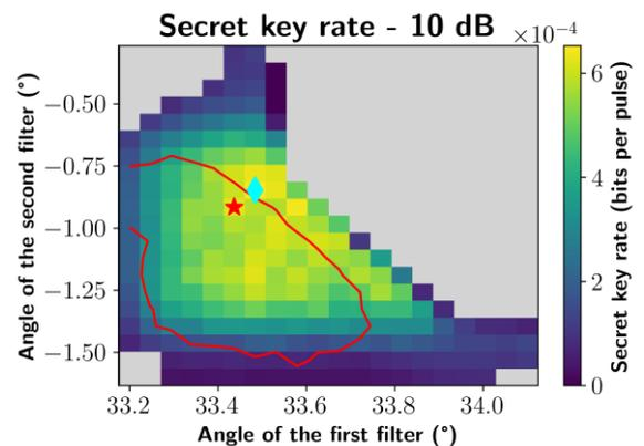
**Figure 1:** SKR as function of the filters' angle. The red region indicates the area where purity is over 95%. The red star marker (resp. blue diamond) indicates the highest SKR in the red region (resp. global maximum).
