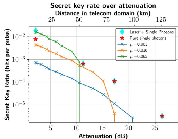
**Figure 2:** Distance scaling of the SKR. Red stars and blue diamonds are data points taken from the SKR colormaps for various attenuations. The SKR measured when only using laser is plotted in coloured lines.
