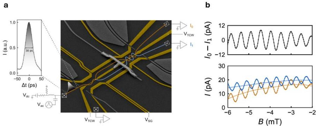
**Fig. 1.** Electronic Mach-Zehnder interferometer with ultrashort wavepackets. (a) Scanning electron micrograph of the electronic MZI. Inset: time-resolved measurement of a 30 ps width wavepacket. (b) Aharonov–Bohm oscillations with a 30 ps wavepacket: the lower panel shows raw data, while the upper panel displays the current difference.
