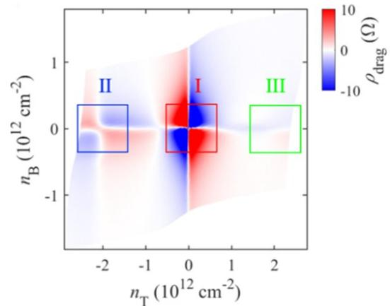
**Figure 2:** Drag resistance as a function of top and bottom graphene density in a color scale. The data were taken at 210 K.
