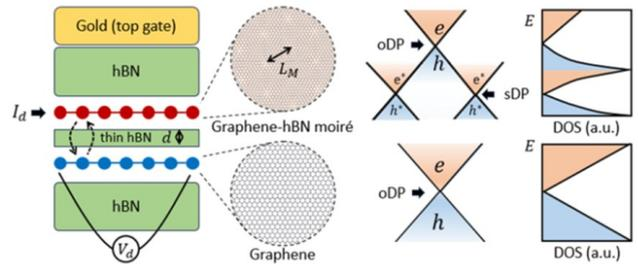
**Figure 1:** Left: Schematic of graphene-hBN-graphene moiré heterostructures and the Coulomb drag measurement configuration. Right: Electronic band structure and density of states (DOS) of graphene-hBN moiré lattice (top) and intrinsic graphene (bottom).
