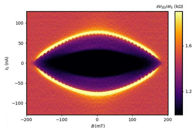
**Figure 2:** Magnetoconductance map of one of the loop devices. Notably, the resistance vanishes for low applied currents and magnetic fields, and Little-Parks oscillations in the critical current can be seen.
