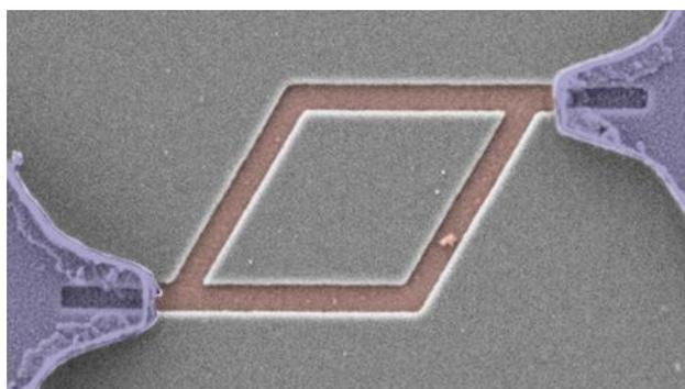
**Figure 1:** False-colored top view SEM image of a selective-area grown tin telluride loop (red) in a silicon nitride mask (grey), with titanium/palladium contacts (purple).
