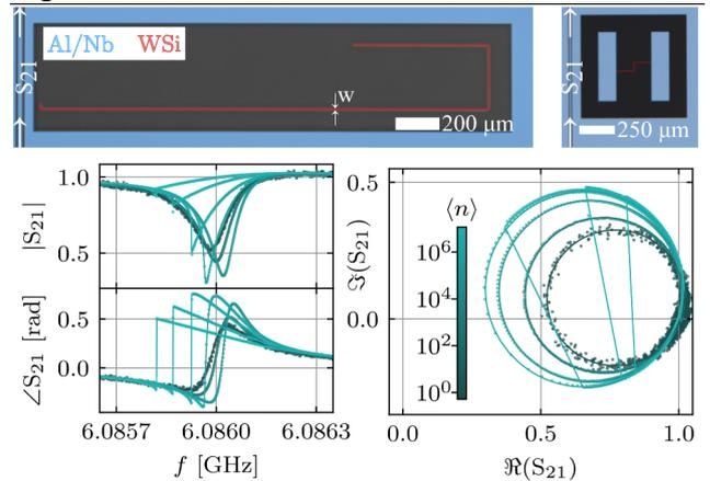
**Figure 1:** False-color optical image of a stripline (top left) and lumped element (top right) style WSi resonator, coupled to the readout feedline. Typical frequency response of a WSi resonator (bottom) at resonator photon numbers. Solid lines are fit to the data.
