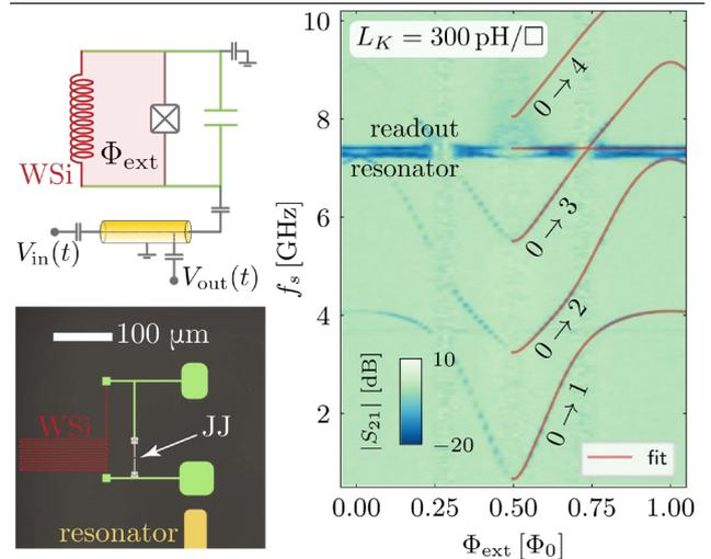
**Figure 2:** Circuit schematic of the investigated WSi fluxonium device (top left) and its false-color optical image (bottom left). Result of a two-tone spectroscopy measurement carried out on a fluxonium with WSi shunt, with nominal film inductance of  $L_K=300$  pH/□. Solid lines are fits according to the Jaynes-Cummings model of the system.
