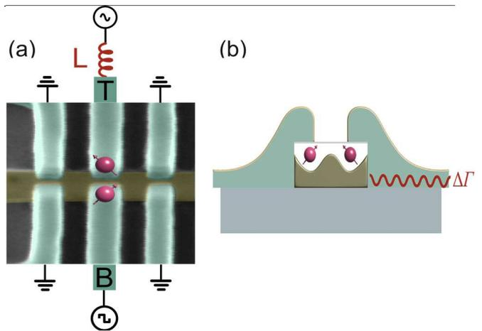
**Figure 1:** (a) Scanning electron microscopy (SEM) with false color showing the device where the qubit unit cell is implemented. (b) Artistic view of a cut of the T-B double dot perpendicular to the channel in (a).
