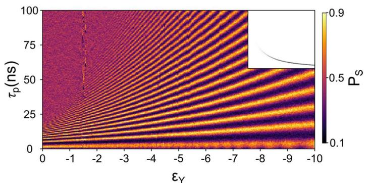
**Figure 2:** Exchange oscillations done at different detunings  $\epsilon_Y$  showing the expected exponential frequency dependency
