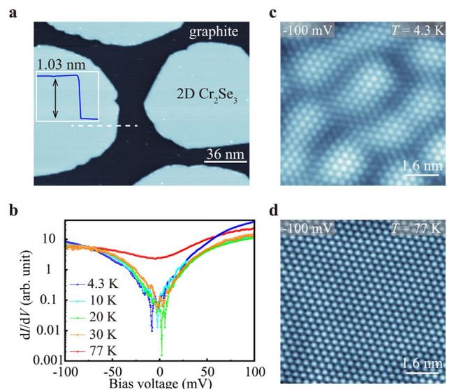
**Figure 1:** (a) STM topographic image of single-layer (SL) Cr<sub>2</sub>Se<sub>3</sub>/graphite. (b) Temperature-dependent dI/dV spectra of SL Cr<sub>2</sub>Se<sub>3</sub>. (c, d) Atomic resolution STM image of SL Cr<sub>2</sub>Se<sub>3</sub> acquired at (c) 4.3 K and (d) 77 K, showing temperature-dependent features.
