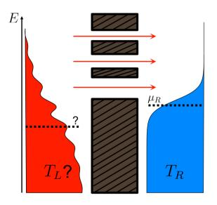
**Figure 1:** A non-thermal electron distribution on the left exchanging energy and particles with a thermal distribution on the right. The brown wall blocks all electrons, while the gaps allow them to flow freely. This type of transmission function gives the highest efficiency for a given input or output.
