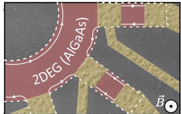
Figure 1: Scanning electron microscopy (SEM) image of the AlGaAs 2DEG device with a zoomed-in false-colour SEM image. The white lines indicate the edge quantum Hall states occurring in the presence of a perpendicular magnetic field at filling factor \nu = 1 , whereas the white arrows indicate the direction of propagation of electrons. The 2DEG and ohmic contacts are highlighted in red and yellow, respectively. The white dashed lines show the boundaries of the 2DEG.
