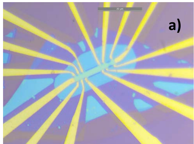
Figure 1: Optical images of two of our typical devices: a) Crenellated channel with a nanoconstriction. b) Tesla valve geometry.
