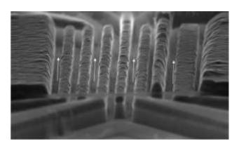
**Figure 1:** SEM imagine of a suspended CNT( indicated by white arrow). The CNT is suspended over 5 electrodes used to define QD.
