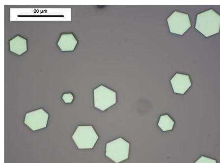
**Figure 1:** Optical image of  $\text{Fe}_x\text{Se}_y$  grown on  $\text{SiO}_2$ .
