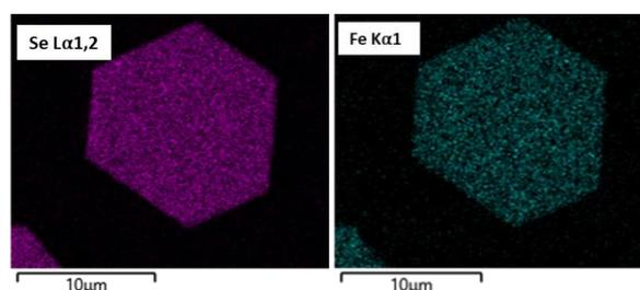
**Figure 2:** EDX map of  $\text{FeSe}$  grown on  $\text{SiO}_2$ .
