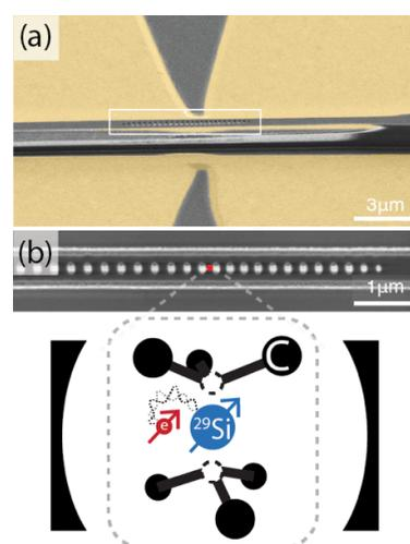
**Figure 1:** (a) SEM of nanobridged optical cavity, waveguide, and gold striplines for MW delivery. (b) Zoomed in section of the cavity. The SiV is located at the optical mode maximum (red dot).
