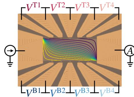
**Figure 1:** An optical micrograph of the QAH Hall bar studied in this work. Eight longitudinal resistance measurements are indicated. A solution of Laplace's equation is superimposed on the Hall bar, matching resistance measurements.
