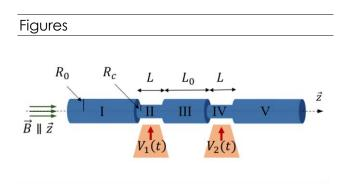
**Figure:** Schematic of the proposed device: a TI nanowire of radius  $R_0$  is etched in regions II and IV, of length L and reduced radius  $R_C < R_0$ , leaving region III of length  $L_0$  in between. Regions I and V are assumed of infinite length. To implement adiabatic quantum pumping, two oscillating electrostatic gates with a nonzero phase difference,  $V_1(t)$  and  $V_2(t)$ , are applied to regions II and IV respectively.
