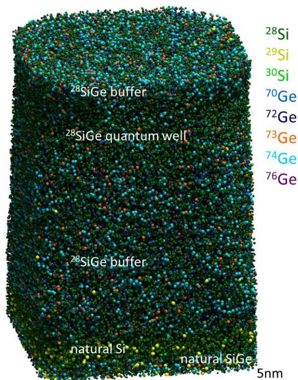
**Figure 1:** Atom Probe Tomography analysis of a quantum well grown sandwiched between silicon germanium buffers grown with <sup>28</sup>Si enriched Silicon.
