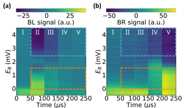
**Figure 2:** Coulomb drag measurement data. (a) Bottom-left and (b) bottom-right sensor signals as a function of time and energy offset of the bottom channel  $E_B$ . In the time domain from II to V an electron is shuttled in the top channel from left to right. As  $E_B$  decreases, a transition from single-electron transport (blue dashed region) to correlated electron-hole pair transport, i.e. exciton transport (orange dashed region), is observed.
