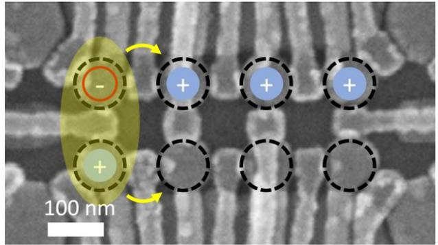
**Figure 1:** A scanning electron microscope image of a germanium 4x2 quantum dot array with a schematic showing excitonic transport. An electron (missing of a hole) is shuttled through the top channel and a hole in the bottom channel is dragged along because of the inter-channel Coulomb interaction.
