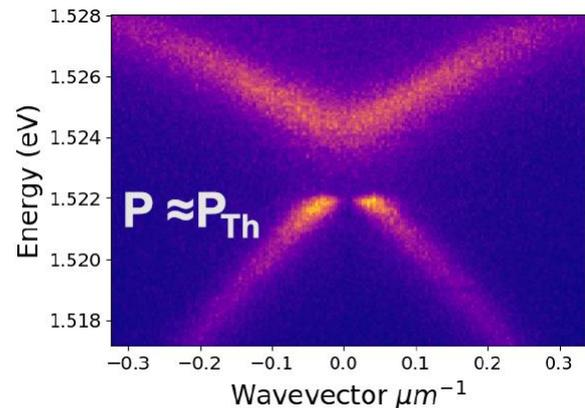
**Figure 2:** Angular resolved PL emission under non-resonant ps (pulsed) excitation (snapshot from a time-resolved streak camera). Around threshold a double peaked emission occurs around  $k \sim 0$ . When the pumping power is increased this emission becomes dominant.
