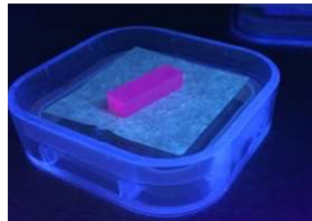
Figure 1: A Tm:Y 3 Ga 5 O 12 crystal used for storing quantum states of light.
