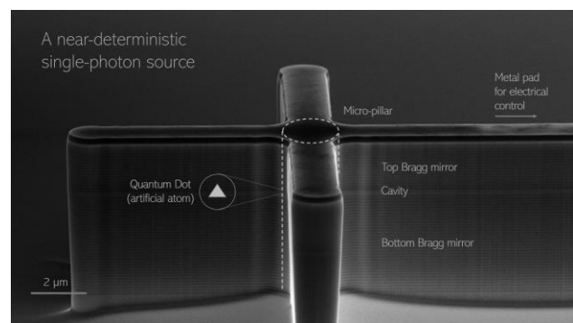
Figure 1: Solid-state quantum light source developed by Quandela
