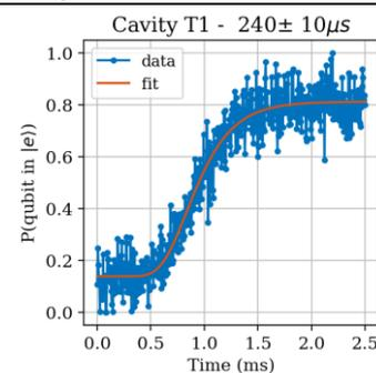
**Figure 2:** High Q Cavity  $T_1$  Measurement – A displacement pulse puts the cavity into a coherent state with high average photon number. The coherent state then decays back to the cavity ground state with characteristic time  $T_1$ , which is probed by a selective  $\pi$  pulse on the qubit transition for the cavity ground state.
