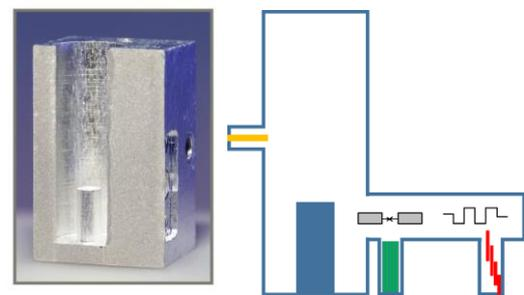
**Figure 1:** (left) Cut picture of a Coaxial cavity. (right) Schematic representation of the setup. SQUID transmons are capacitively coupled to the High Q Coaxial Niobium cavity. The SQUIDs are tuned with a Flux Hose and protected by a Purcell Filter, which is integrated into the readout pin.
