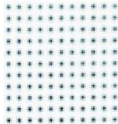
Figure 1: Array of Strontium atoms in optical tweezers
