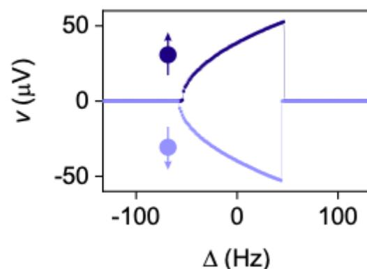
**Figure 2:** Measured out-of-phase response  $v$  of the resonator to parametric driving as a function of detuning.
