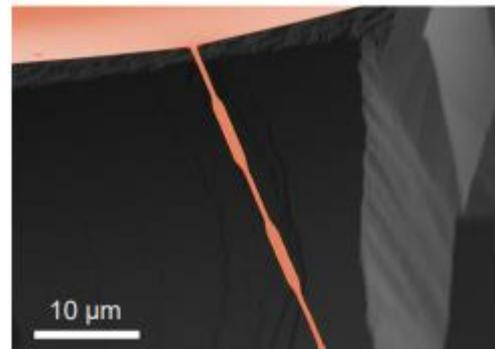
**Figure 1:** A false-colored SEM image of a high- $Q$  nanomechanical string device. Shown is one clamping point and two unit cells.
