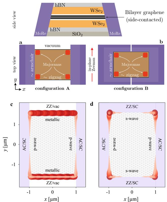
**Figure 1:** Top and lateral views of the proposed device configurations A and B (a-b). Spatial density of Majorana delocalised zero modes (c) and Majorana bound states (d) on top of the lattice.
