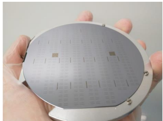
Figure 1: Photograph of a 100 mm wafer containing more than 5,000 connected silicon nanowires
