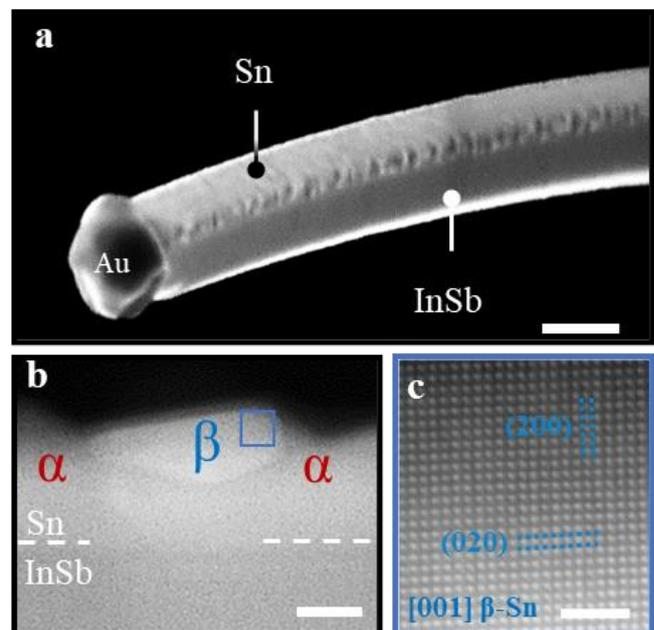
**Figure 1:** Electron microscopy analysis of one hybrid InSb-Sn nanowire sample of our study.
