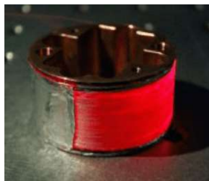
Figure 2: An experimental sample of thulium-doped yttrium gallium garnet (Tm: YGG) which could serve as a photon memory. (The picture is adapted from: https://qutech.nl/lab/tittel-lab/tittel-lab-research-overview/quantum-memory/ )
