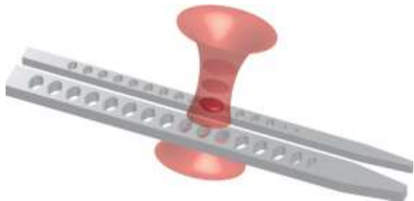
Figure 1: The optical-trapped cold Rb atom (solid red dot) that is designed to emit two entangled photons. Thus, it is coupled to two nanophotonic cavities of different resonance frequencies.
