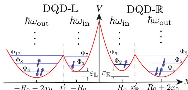
**Figure 1:** Schematic illustration of a double double-quantum-dot (DQD) device, where DQD-L and -R denote left and right DQD respectively, with  $x = 0$  being the boundary between them.
