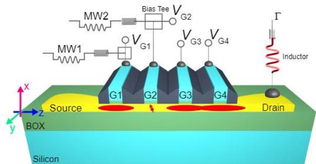
**Figure 1:** Simplified 3-dimensional representation of a silicon (yellow)-on-insulator (green) nanowire device with four gates. Gate 2 (G2) defines a quantum dot hosting a single hole. The drain contact is connected to an off-chip, surface-mount inductor to enable rf-reflectometry readout.
