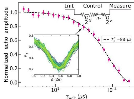
**Figure 2:** Normalized echo amplitude versus the free evolution time using a Hahn echo sequence (See top left inset). Black dashed line represents the Gaussian fit to extract the extended coherence time at the optimised working point.
