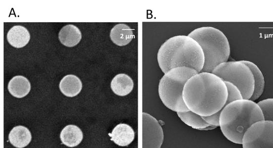
SEM images, (A) microdisks adhered to Si substrate, step 4 and (B) microdisks released in suspension, step 5.
