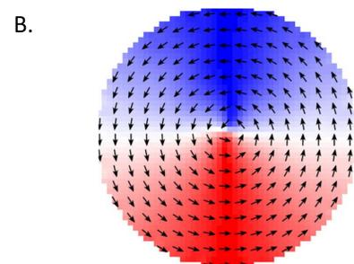
Magnetic characterization: (A) SQUID hysteresis loop of microdisks (diameter 3.4 mm and thickness 100 nm) attached to the substrate (step 4). (B) Representative illustration of the vortex state at zero field.
