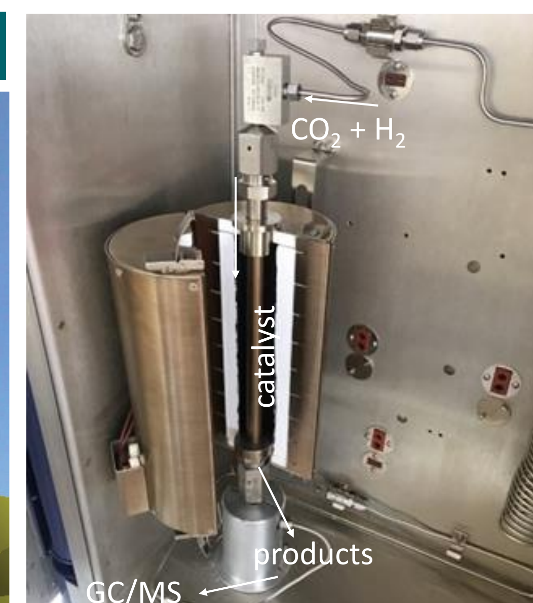
Fig. 4 Microreactor Microactivity Effi (inside) and scheme of the experiment.
