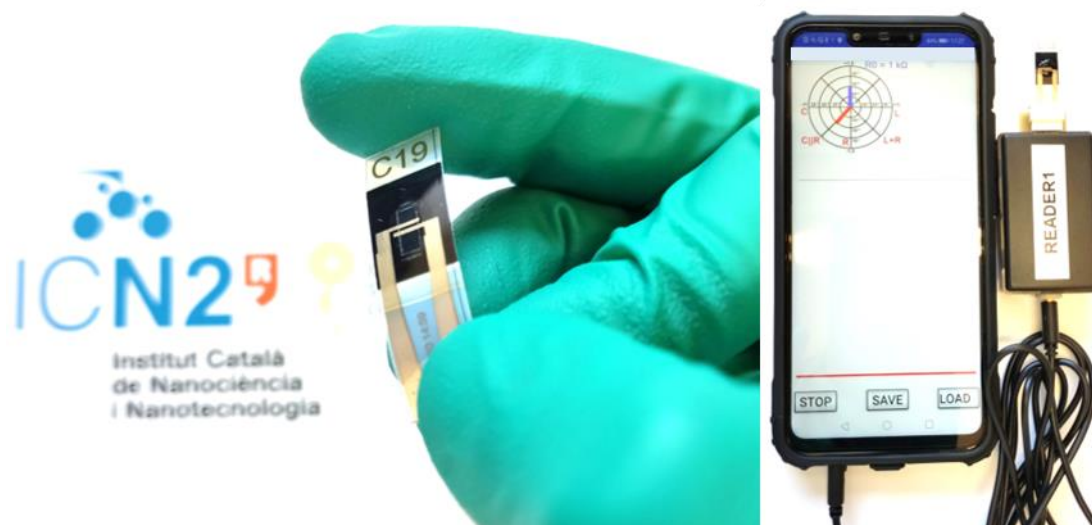
Figure 1: Inkjet printed impedimetric nanobiosensor for the SARS-CoV-2 SP detection with smartphone readout.
