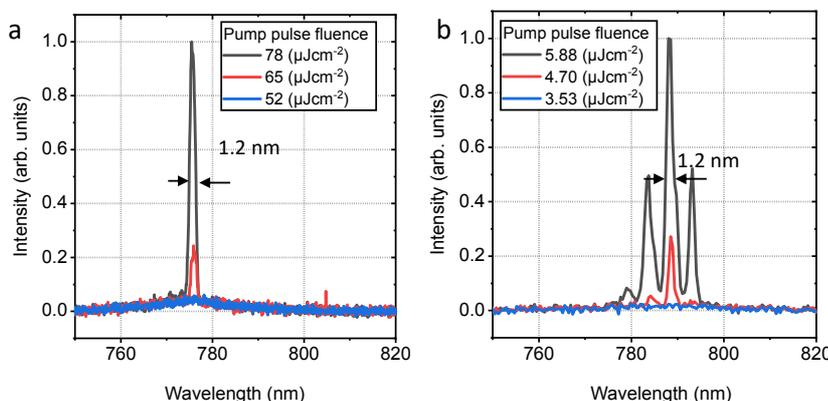
**Figure 2:** a) Laser spectrum obtained by pumping with 700 ps pulses at 532 nm wavelength b) Laser spectrum obtained by pumping with 120 fs pulses at 630 nm wavelength
