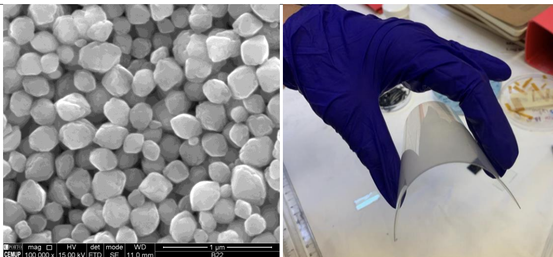
Figure 1: SEM image of hematite nanoparticles deposited on the Flexible ITO/PET substrate.
