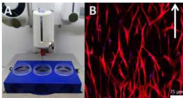
**Figure 1.** A) Image of the experimental setup used for magnetically- and matrix-assisted 3D bioprinting procedures. B) Confocal microscopy image of elongated hASCs aligned in the direction dictated by the sMRFs oriented within anisotropic polymeric hydrogels.
