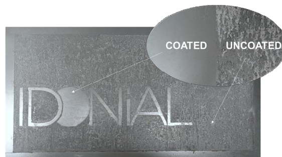
Figure 1. Protective effect of SiO x _Ni-NWs sol-gel coating on DX51D+Z galvanised steel
