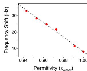
**Figure 3.** Mechanical resonance frequency shift produced when 200 V at 100 kHz voltage is applied on the electrodes for samples of different electric permittivity.
