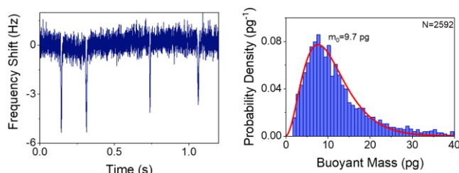
**Figure 2.** (left) Resonance frequency shift produced by the pass of 4 *S. cerevisiae* cells and (right) cell mass distribution obtained for a whole sample.
