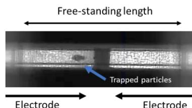
**Figure 1.** Microscope image of the developed device containing a cluster of immobilized particles by dielectrophoretic forces.
