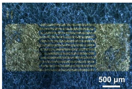
Figure 1: Optical micrograph of a WS 2 photodetector on paper. Figure 2: Photoreponse performance of the WS 2 device.
