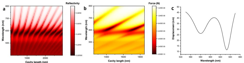
**Figure 2:** a. Reflectivity (in color) as a function of the illuminating wavelength (y-axis) and the cavity length (x-axis). b. Optical Force calculated as a function of the wavelength and the cavity length. c. Relative mechanical displacement of the mechanical structure placed 1500 nm over the reflecting substrate as a function of the wavelength of the pump laser.
