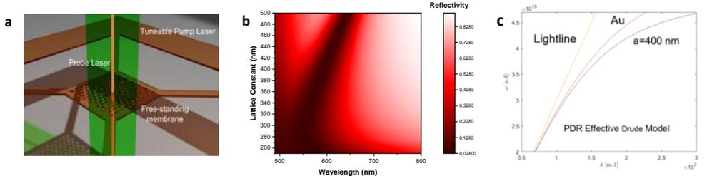
**Figure 1:** a. Schematic depiction of the optomechanical system. b. Color map of the membrane reflectivity as a function of the lattice constant of the nanohole arrays and the illuminating wavelength. The excitation of the Surface Plasmon Polariton is viewed as a reflectivity drop. c. Surface Plasmon dispersion relation calculated by an Effective Drude Model.
