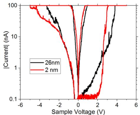
**Figure 2:** I/V RS curves of 2 nm and 26 nm SrIrO<sub>3</sub> thin films.
