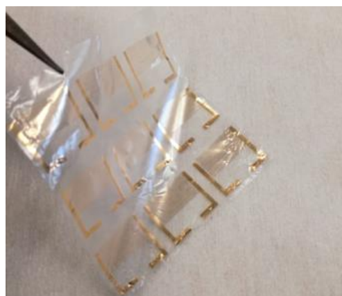
Figure 2. Graphene biosensors printed on polymer.
