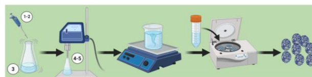
Figure 1. Fabrication of PLGA particles, with 5 steps to control their size, and so degradation and lactate release. (1) Polymer concentration + molecular weight (high (HMw) vs low (LMw)), (2) Lactide monomer concentration, (3) PVA concentration, (4) Intensity of ultrasonication, and (5) Duration of sonication.
